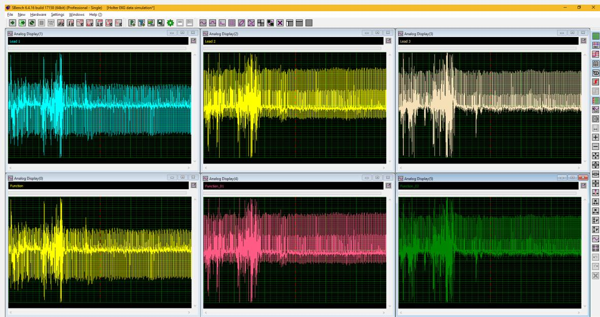
**Figure 4:** An example of an record and replay test strategy using a three wire Holter ECG recorder. The three upper traces are acquired from leads 1 through 3. The signals are copied and replayed three AWG's channels.
