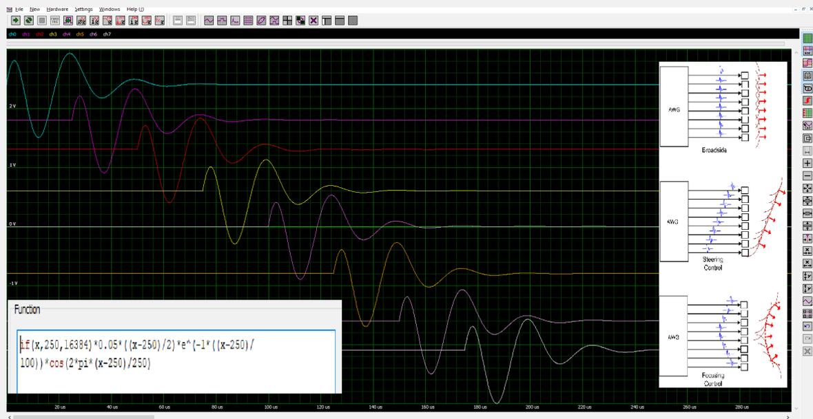
**Figure 7:** Eight ultrasonic waveforms each with a delay of 25  $\mu$ s from the previous one are created using eight equations, one of which is shown in the insert on the lower left of the figure. The other insert shows possible steering or focusing opportunities based on the programmed delay of each waveform.
