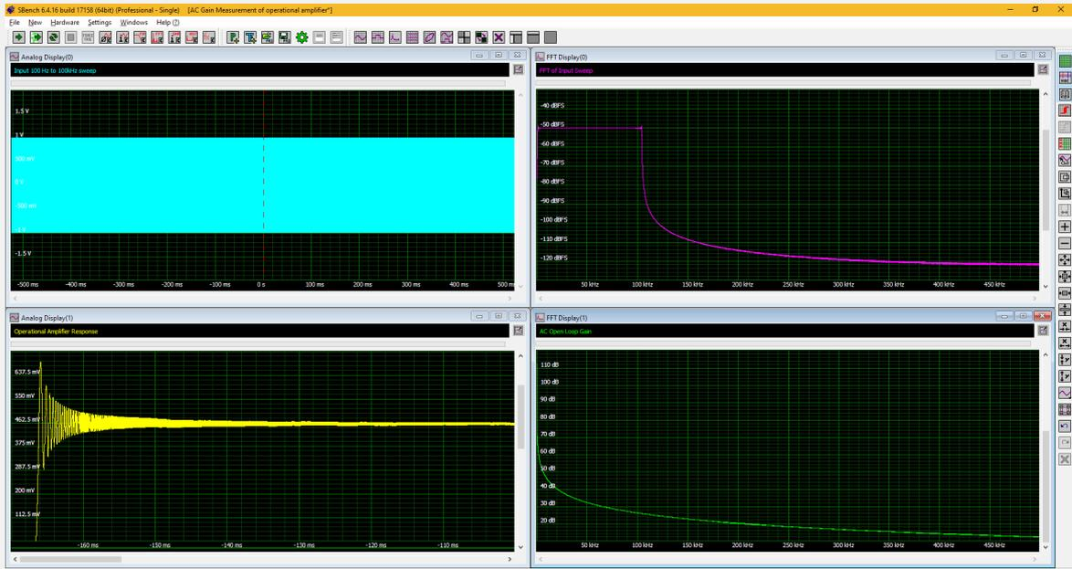
**Figure 3: The four major steps in the AC open loop gain measurement. Signal generation (upper left), input signal frequency range verification (upper right), output signal acquisition (lower left) and frequency response extraction from the output signal (Lower right) which is the AC open loop gain.**
