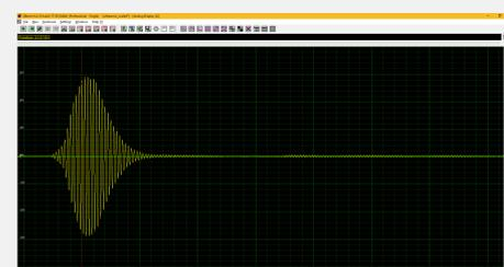
Figure 6: A transmitted ultrasonic pulse and multiple reflected echoes.
