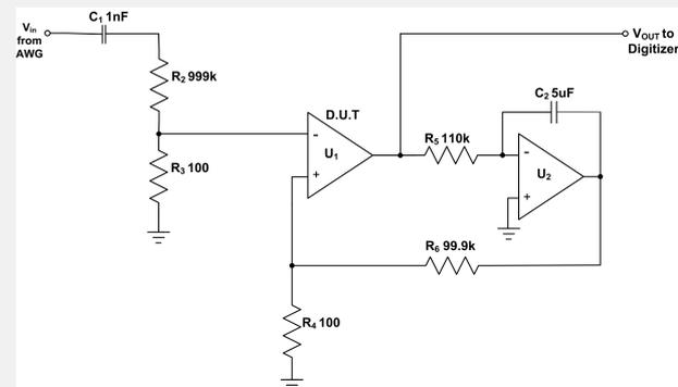
Figure 2: The test circuit for measuring the AC open loop gain of an operational amplifier using an AWG as the source and a digitizer for the response measurement.
