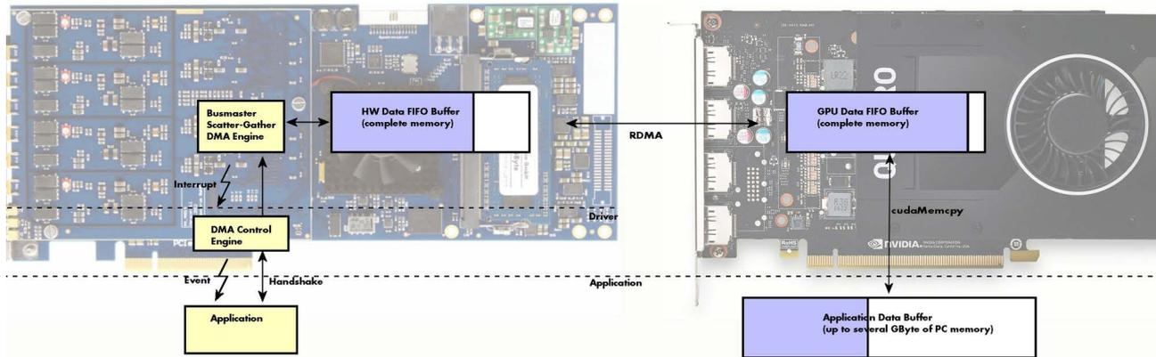
Buffer handshaking for DMA transfer from Spectrum Digitizer to GPU (or vice versa) using RDMA uses the same registers as the transfer from Digitizer to host (or host to Generator) as described in the „Buffer handling” section of the hardware manual.
