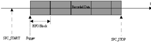
The FIFO mode allows to record data continuously and transfer it online to the PC (acquisition boards) or allows to write data continuously from the PC to the board (generation boards). Therefore the on-board memory of the board is used as a continuous buffer. On the PC the data can be used for any calculation or can be written to hard disk while recording is running (acquisition boards) or the data can be read from hard disk and calculated online before writing it to the board.
