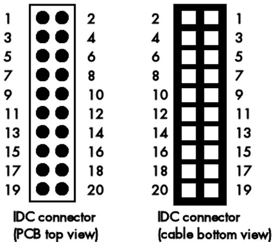
The 20 pole IDC connectors have the following footprints. For easy usage in your PCB the cable footprint as well as the PCB top footprint are shown here. Please note that the PCB footprint is given as top view.
