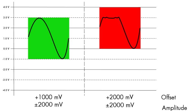
**To avoid heavily distorted output signals please make sure to keep the signals in a range of  $\pm 3000$  mV.**
