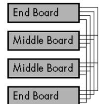
When synchronizing multiple boards, one is set to be the clock master for all the connected boards. All the other boards are working as clock slaves. It's also possible to temporarily disable boards from the synchronization.
