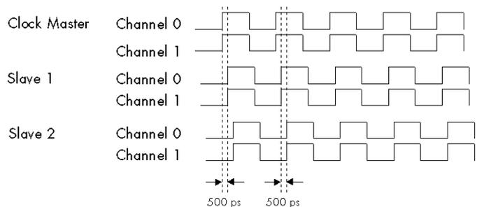
Please keep in mind that the delay between the channels of two boards is depending on which board is actually set up as the clock master and what boards are directly adjacent to the master.
