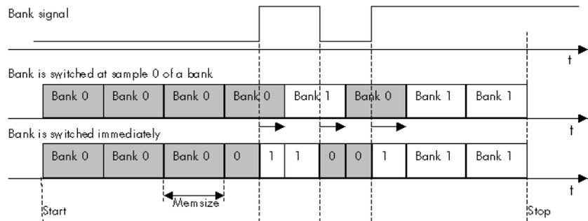
**The data of the two different output signals are stored in multiplex format. For this reason the output signal on the dedicated channel is only updated with half of the programmed sample rate, when bank switching mode is enabled.**
