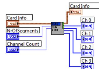
Requires the Signal Processing Firmware option: Block Statistic (M4i.xxxx-spstat) to be installed on the card.
