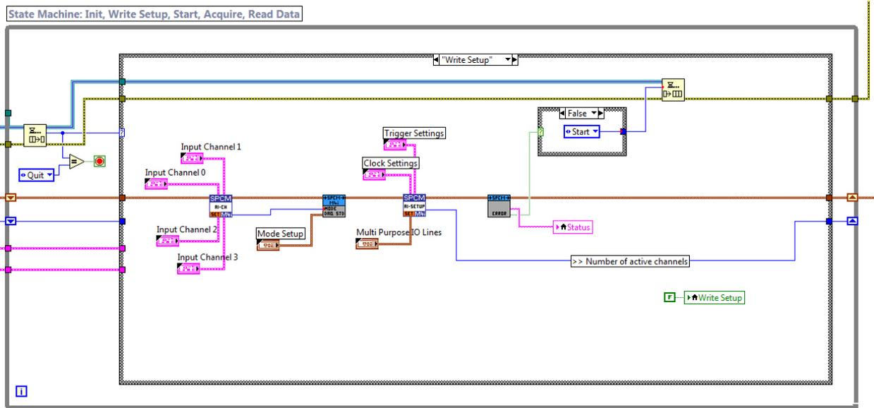
There are different states, such as „Write Setup“ or „Read Data“ that will be processed in a certain order to do an acquisition or generation of data.
