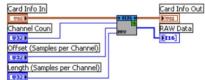
This VI can be used with FIFO mode as well as with standard mode. In FIFO mode it will read out the next free block of data, in standard mode it will read some data directly from the on-board memory.
