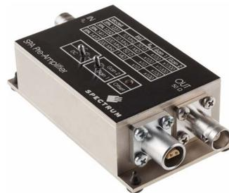
For the acquisition of extremely small voltage levels with a high bandwidth a series of external amplifiers is available. Each of the one channel amplifiers is working with a fixed input impedance and allows - depending on the bandwidth - to select different amplification levels between x10 (20 dB) up to x1000 (60 dB). Using
