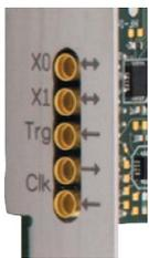
All M3i cards offer two universal multi-purpose I/O lines, which can be separately programmed as either input or output. These lines can be used as additional TTL trigger inputs for more complex trigger conditions. When used as outputs, these lines can be used to output card status signals like trigger-armed or to output the trigger to synchronize external equipment.
