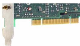
The cards with PCI/PCI-X bus connector use 32 Bit and up to 66 MHz clock rate for data transfer. They are 100% compatible to Conventional PCI > V2.1. The universal interface allows the use in PCI slots with 5 V I/O and 3.3 V I/O voltages as well as in PCI-
