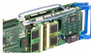
The star-hub is an additional module allowing the phase stable synchronization of up to 8 boards of a kind in one system. Independent of the number of boards there is no phase delay between all channels. The star-hub distributes trigger and
