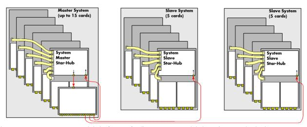
The master system generates trigger and clock information for all systems. Trigger and clock signals are routed to the slave systems as well as to the master itself using shielded coax cables. The system-connection lines have equal length. Within each system a System Star-Hub distributes the signals to each connected card. These cables again have all the same length.
