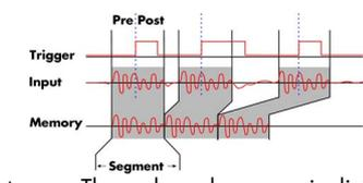
The Multiple Recording mode allows the recording of several trigger events with an extremely short re-arming time. The hardware doesn't need to be restarted in between.
