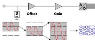
The analog inputs can be adapted to real world signals using a wide variety of settings that are individual for each channel. By using software commands one can select a matching input range
