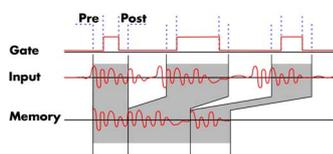
The Gated Sampling mode allows data recording controlled by an external gate signal. Data is only recorded if the gate signal has a programmed level. In addition a pre-area before start
