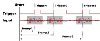
The timestamp function writes the time positions of the trigger events in an extra memory. The timestamps are relative to the start of recording, a defined zero time,
