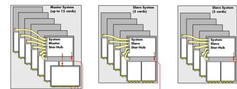
With the help of multiple system star-hubs it is possible to link up to 17 system phase synchronous with each other.
