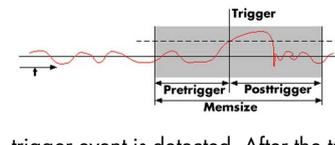
The ring buffer mode is the standard mode of all oscilloscope instruments. Digitized data is continuously written into a ring memory until a
