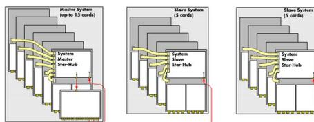
With the help of multiple system star-hubs it is possible to link up to 17 system phase synchronous with each other. Each system can then contain up to 16 cards (master only 15). In total 271 cards can be used fully synchronously in a bunch of systems. One master system distributes clock and trigger signal to all connected slave systems.
