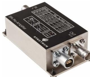
For the acquisition of extremely small voltage levels with a high bandwidth a series of external amplifiers is available. Each of the one channel amplifiers is working with a fixed input impedance and allows - depending on the bandwidth - to select different amplification levels between x10 (20 dB) up to x1000 (60 dB). Using the external amplifiers of the SPA series voltage levels in the uV and mV area can be acquired.
