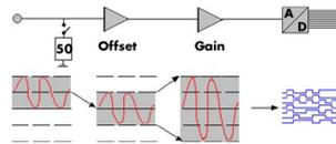
The analog inputs can be adapted to real world signals using a wide variety of settings that are individual for each channel. By using software commands the input termination can be changed
