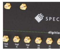
Standard SMA connectors are used for all analog input signals and all trigger and clock signals. No special adapter cables are needed and the connection is secure even when used in a moving environment.
