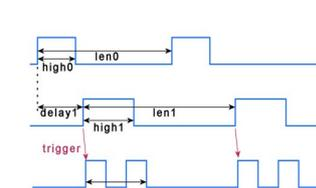
The digital pulse generator option adds 4 internal independent digital pulse generators with programmable duty cycle, output frequency, delay and number of loops. These digital pulse generators can be triggered by software, hardware trigger or can trigger
