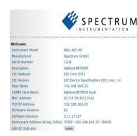
The integrated webserver follows the LXI standard and gathers information on the product, set up of the Ethernet configuration and current status. It also allows the setting of a configuration password, access to documentation and updating of the complete instrument firmware, including the embedded remote server and the webserver.
