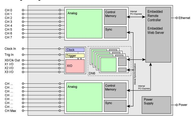
• The number of maximum channels and internal AWG modules and existance of a synchronization Star-Hub is model dependent.
