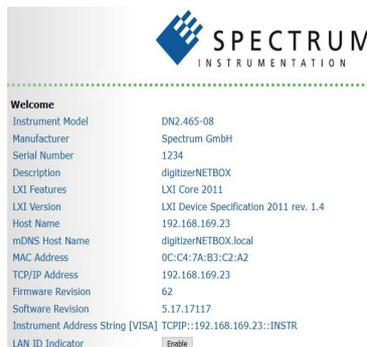
The integrated webserver follows the LXI standard and gathers information on the product, set up of the Ethernet configuration and current status. It also allows the setting of a configuration password, access to documentation and updating of the complete instrument firmware, including the embedded remote server and the webserver.
