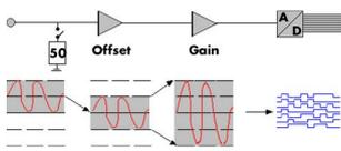
The analog inputs can be adapted to real world signals using a wide variety of settings that are individual for each channel. By using software commands the input termination can be changed between 50 Ohm and 1 MOhm, one can select a matching input range and the signal offset can be compensated for.
