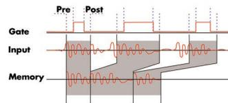
The Gated Sampling mode allows data recording controlled by an external gate signal. Data is only recorded if the gate signal has a programmed level. In addition a pre-area before start of the gate signal as well as a post area after end of the gate signal can be acquired. The number of gate segments is only limited by the used memory and is unlimited when using FIFO mode.
