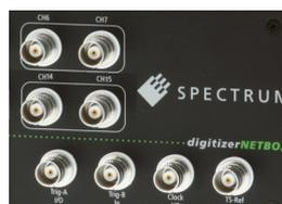
Standard BNC connectors are used for all analog input or output signals and all auxiliary signals like clock and trigger. No special adapter cables are needed and the connection is secure even when used in a moving environment.
