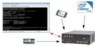
The option turns the digitizerNETBOX/generatorNETBOX in a powerful PC that allows to run own programs on a small and remote data acquisition system. The digitizerNETBOX/generatorNETBOX is enhanced by more memory, a powerful CPU, a freely accessible internal SSD and a remote software development access method.
