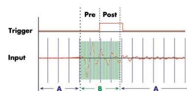
The ABA mode combines slow continuous data recording with fast acquisition on trigger events. The ABA mode works like a slow data logger combined with a
