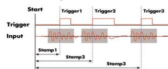
The timestamp function writes the time positions of the trigger events in an extra memory. The timestamps are relative to the start of recording, a defined zero time, externally synchronized to a radio clock, an IRIG-B a GPS receiver.
