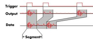
The Multiple Replay mode allows the fast output generation on several trigger events without restarting the hardware. With this option very fast repetition rates can be achieved. The on-board memory is divided into several segments of the same size. Each segment can contain different data which will then be played with the occurrence of each trigger event.
