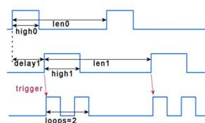
The digital pulse generator option adds 4 internal independent digital pulse generators with programmable duty cycle, output frequency, delay and number of loops.
