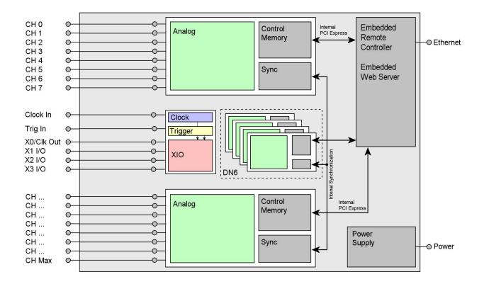
• The number of maximum channels and internal AWG modules and existance of a synchronization Star-Hub is model dependent.
