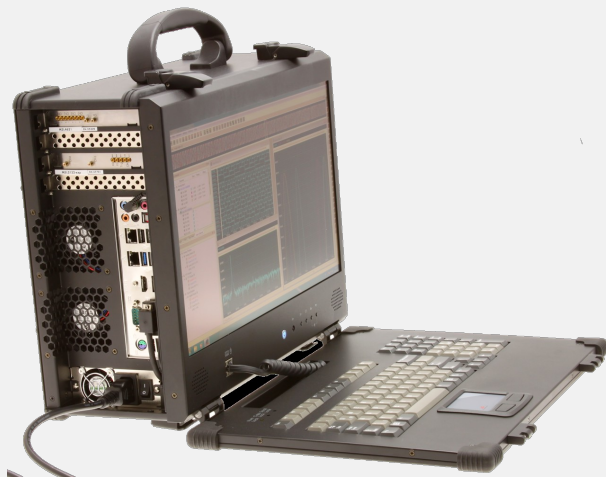
Figure 1: A portable computer serves as the chassis for dual PCIe based digitizers creating a mobile test system.
