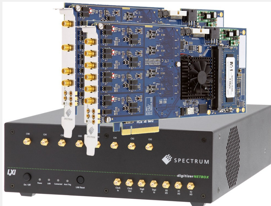
Spectrum's PCIe and LXI digitizers include the necessary hardware and software features needed to perform like an oscilloscope
