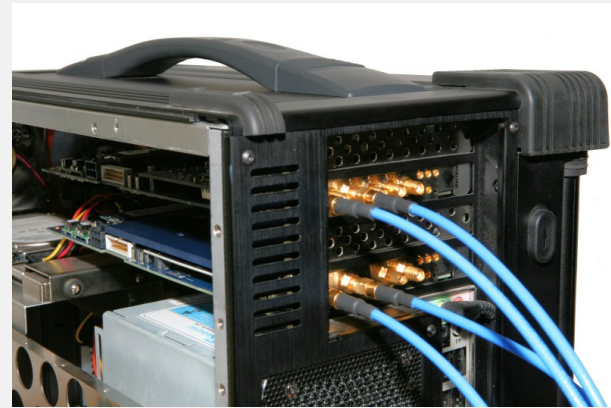
Figure 1: A typical modular stimulus-response test system composed of Spectrum M4i.4451-x8, 500 MS/s, 250 MHz, 14-bit digitizer and an M4i.6631-x8, 1.25 GS/s, 400 MHz, 16 bit, arbitrary waveform generator mounted in a portable computer.
