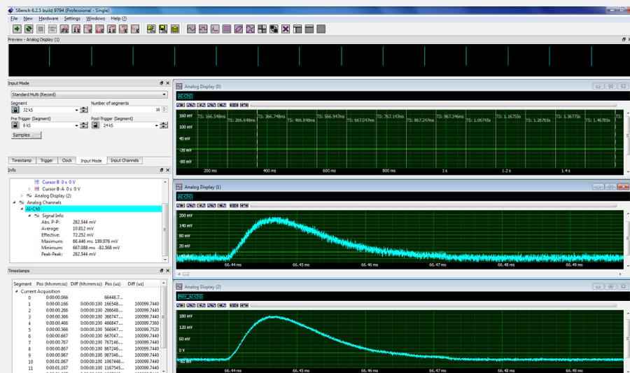
Figure 2: Segmented acquisition of a simulated laser pulse with short pulses and long dead time
