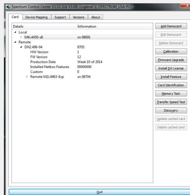
Figure 3: The Discovery function of the Spectrum control center finds all instances of the digitizerNETBOX available to the computer
