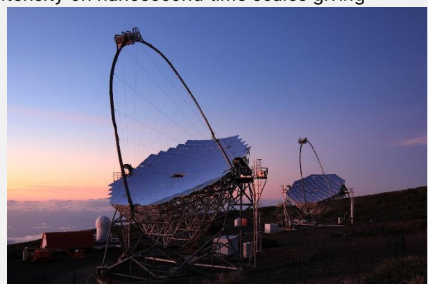
Figure 2: MAGIC (Major Atmospheric Gamma-Ray Imaging Cherenkov) are the world's largest air-Cherenkov-telescopes each with a diameter of 17m
