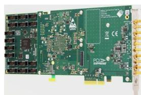
The Star-Hub is an additional module allowing the phase stable synchronization of up to 16 boards in one system. Two versions are available: one with up to 6 cards and the large version supports up to 16 cards in one system. Both versions can be mounted in two different ways, to either extend the cards
