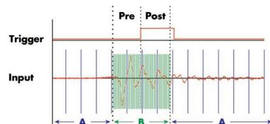
The ABA mode combines slow continuous data recording with fast acquisition on trigger events. The ABA mode works like a slow data logger combined with a
