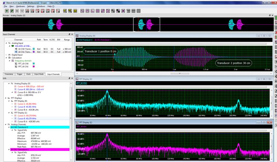
Figure 1: SBench 6, a Powerful, Interactive Software Tool for Acquiring and Analyzing Digitizer Data
