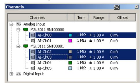
Using the right mouse on the channel selection will open a context menu which allows to select the enable/disable state of the selected channel as well as some other settings. The current activation state is shown by a check next to the enable/disable command.
