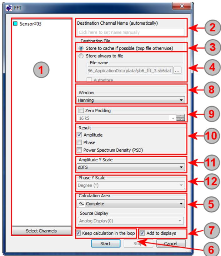
1 This area shows the selected signals for the calculation. Each calculation can be issued for one or several signals, each running the calculation independent then. To modify the list of source signals the „Select Channels“ button can be used.
