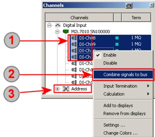
1 All signals that should be combined are marked with the mouse. One bus can combine at maximum up to 64 digital channels.
