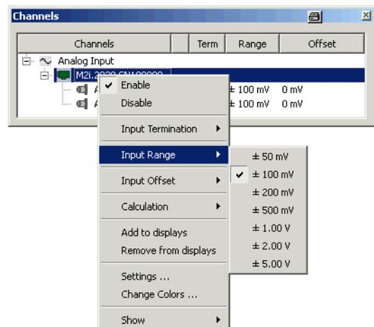
The currently selected setting is shown with a check if all channels are actually set to the same setting. If the channels have different settings no check is shown. Clicking on one setting will of course then change all channels to use the same setup.
