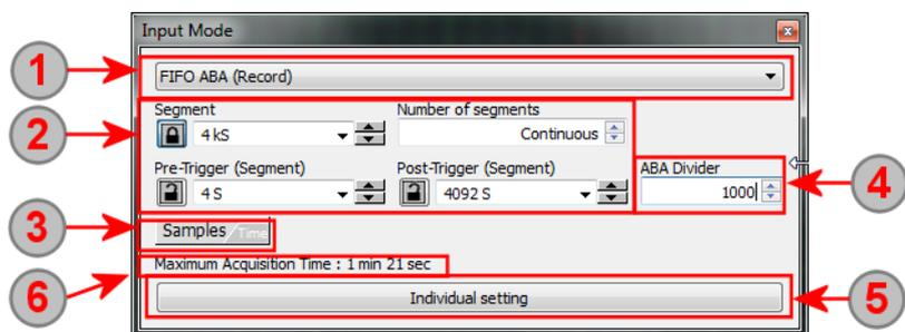
One can select one of the pre-defined values from the drop-down list of the field or one can enter any value directly into the field. SBench 6 will then change this value automatically to the nearest matching value taking the modifier into account as shown under (3). A third method of entering values is the usage of the up/down buttons just right next to the field. These buttons will go step by step through the valid values of this field and allow a very fine tuning of the memory settings.
