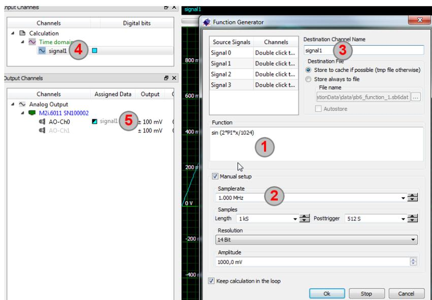
5 By dragging the generated time domain signal to the output channel you set the connection and define this signal to be used as an output signal for this channel.
