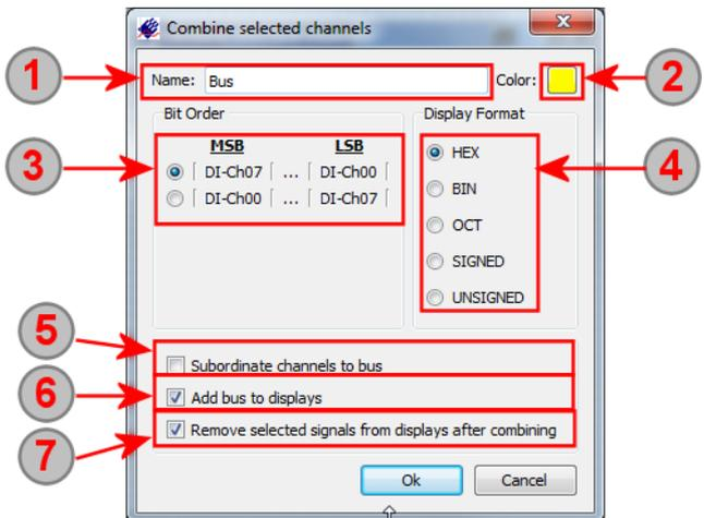
1 A name can be given to the signal that defines the bus and that is used in the digital display window.
