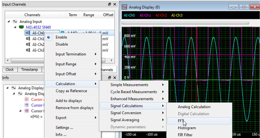
The same FFT calculation can be found if going through the menu „New“. In here the analog signals for which the FFT calculation should be done must be selected manually.
