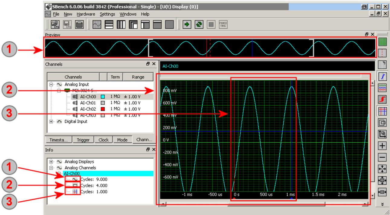
1 Complete signal area, shown in the calculation results as . In here the complete signal is used for the calculation independent of the current display view or the cursor position. In our example the complete signal has 9 full signal cycles which is shown as a calculation result in the information window under (1).
