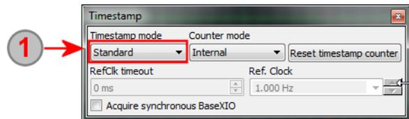
If Gated Sampling is activated the timestamp information is needed to show segmented information. Multiple Recording signals can also be shown without timestamp information just showing the segment borders with no time position information then.
