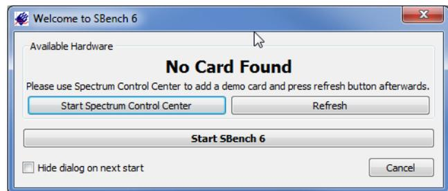
Therefore one starts the „Spectrum Control Center“ that has been installed together with SBench 6 and the needed driver libraries. The Control Center can be started directly from the SBench 6 welcome dialog.
