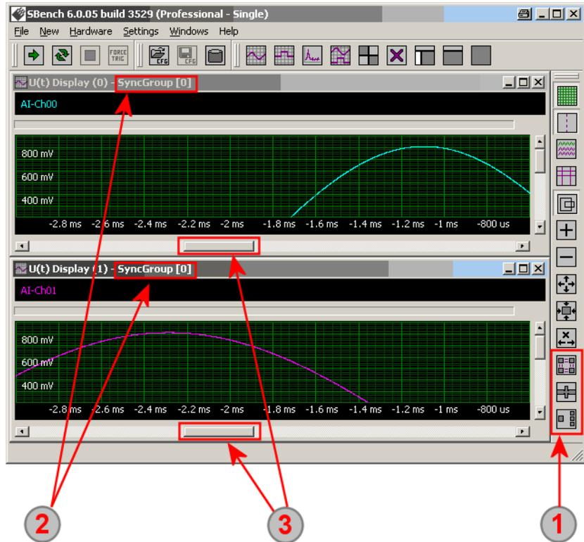
1 The icons handle the display synchronization and allow to set up synchronization, to split up the displays or to temporarily take one display from synchronization.
