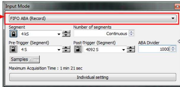
Please note that there is no segmented view if using Gated Sampling with no Timestamps activated. As the length of the gates is depending on an external signal SBench 6 has to know the length of the gate signals by acquiring timestamps to show any segment information then.
