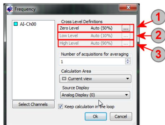
The crosslevel setup allows to either program the crosslevel relatively or absolute:
