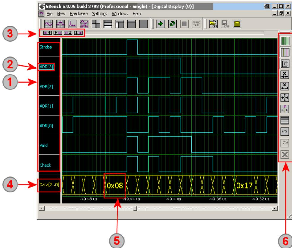
1 Single signals are shown with their name as defined inside the channel dialog. See the next chapter to see how to sort signals inside the display.
