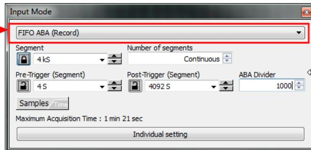
Please note that there is no segmented view if using Gated Sampling with no Timestamps activated. As the length of the gates is depending on an external signal SBench 6 has to know the length of the gate signals by acquiring timestamps to show any segment information then.
