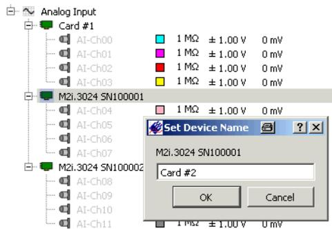
When using several cards in one system it is useful to change the names of the cards according to the used cabling. A simple example may be to just number all cards in a system from left to right to know which channel is located where at the connection panel. Unfortunately the PC itself doesn't give a defined location info. As a default SBench 6 is showing the card type and the serial number as a device name. This can be changed to any name that may be suitable for the user.
