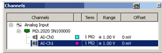
It is also possible to mark multiple channels to access the setting of multiple channels at the same time with the mouse wheel. Marking multiple channels is explained above. Please note that you need to mark the channel at the position of the setting that you like to change afterwards.
