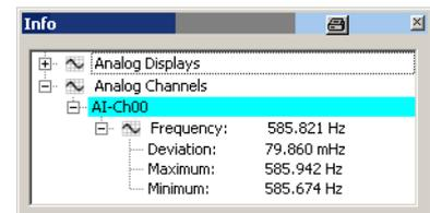
In our example we see a very small frequency variation throughout our analyzed signal and see that the signal is only varying between 585.674 Hz and 585.942 Hz with an average frequency of 585.821 Hz and a very small deviation (difference from the average value) of only 79.860 mHz.
