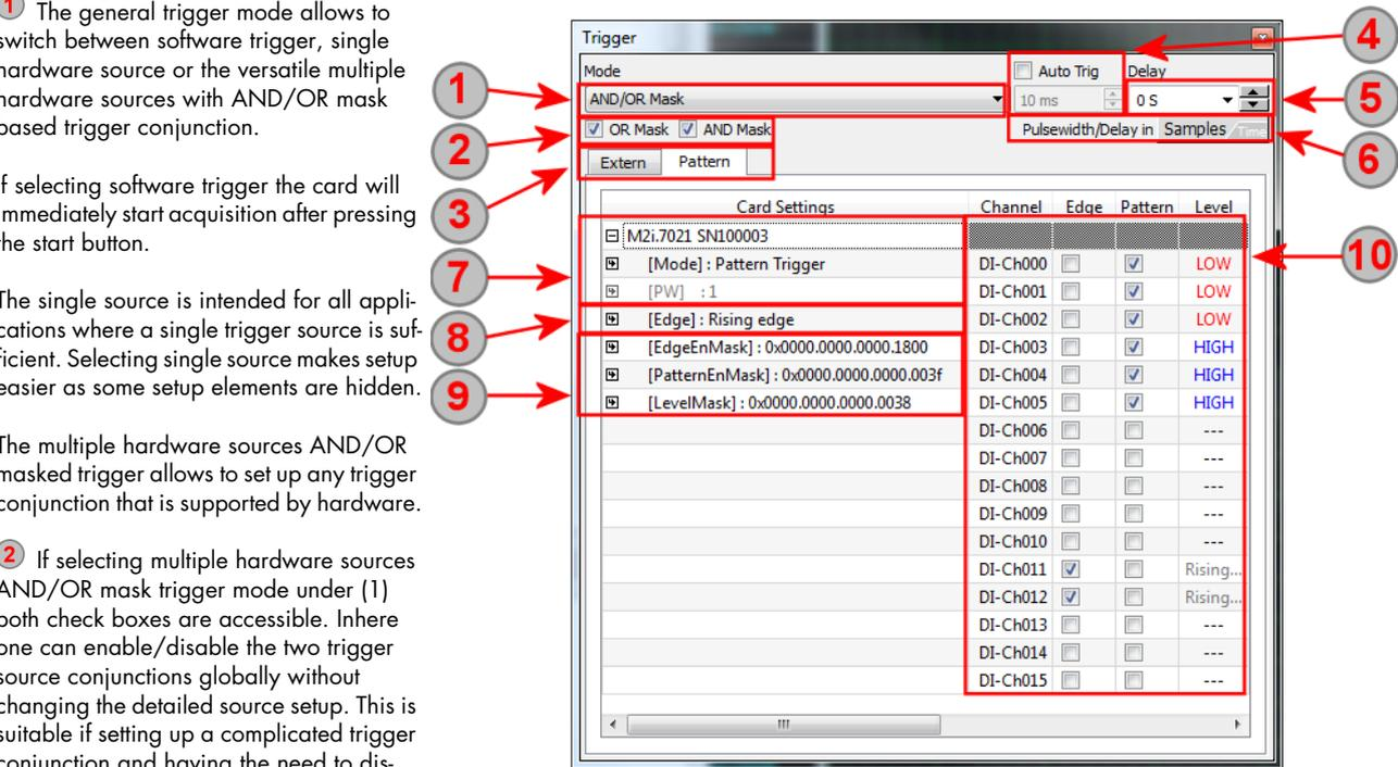
64 kS  If selected to samples input the field will accept pure samples values or entries with a samples modifier input of „k“, „M“, „G“:
