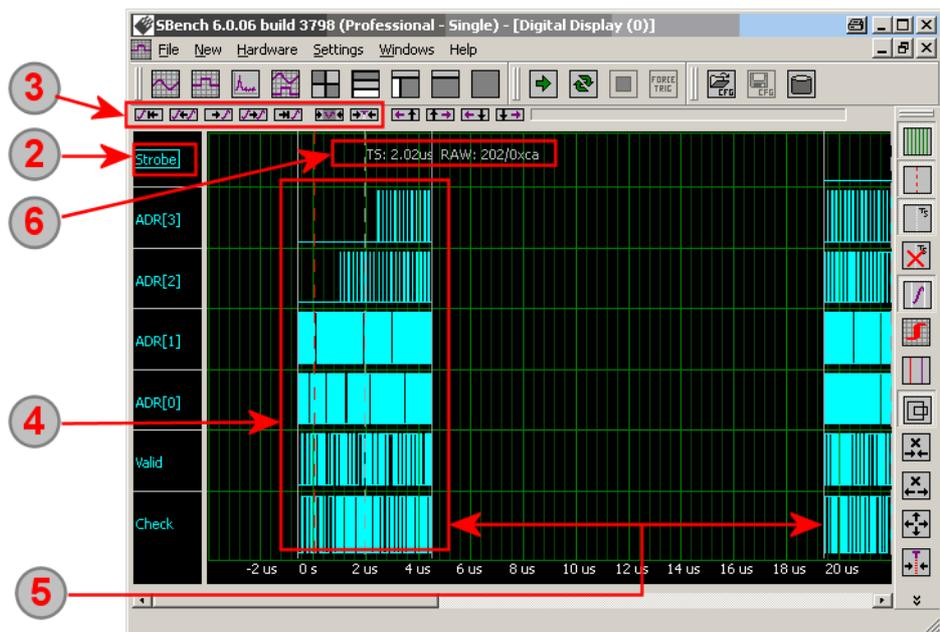
(3) If a signal is marked as source for segment control as shown under (2) these additional segment control buttons appear. The segment control buttons can also be added to the toolbars by just using the standard toolbar editing functions. The control buttons are explained in further detail in the next chapter.
