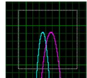
In this mode the mouse can be used to define the exact area to which one wants to zoom. The area is defined by moving the mouse over the area of interest with the left mouse button pressed. After releasing the mouse button the display will zoom into the freshly defined area.
