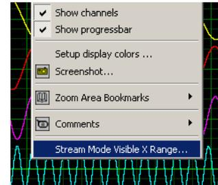
The stream mode settings define the FIFO preview setup for the current display. It is possible to have different FIFO preview displays having different stream mode settings.
