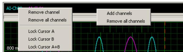
Channels can be either removed by issuing the „Remove all channels“ command or by right clicking on a single channel and issuing the „Remove channel“ command. Multiple channels can also be removed by marking all of them with the CTRL key and left mouse button and then right clicking on one of the channels calling the „Remove channel“ command.
