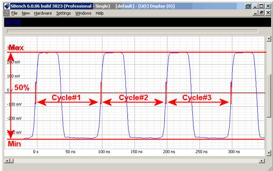
After the exact cycle transitions have been detected each cycle is determined for himself calculating the figures of interest for each cycle.
