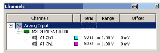
If channels have different settings at the beginning the first turn of the mouse wheel will change the setting of the first channel to the next setting and will automatically set all other channels to the same setting. Starting with the second mouse turn all channels will change settings simultaneously.
