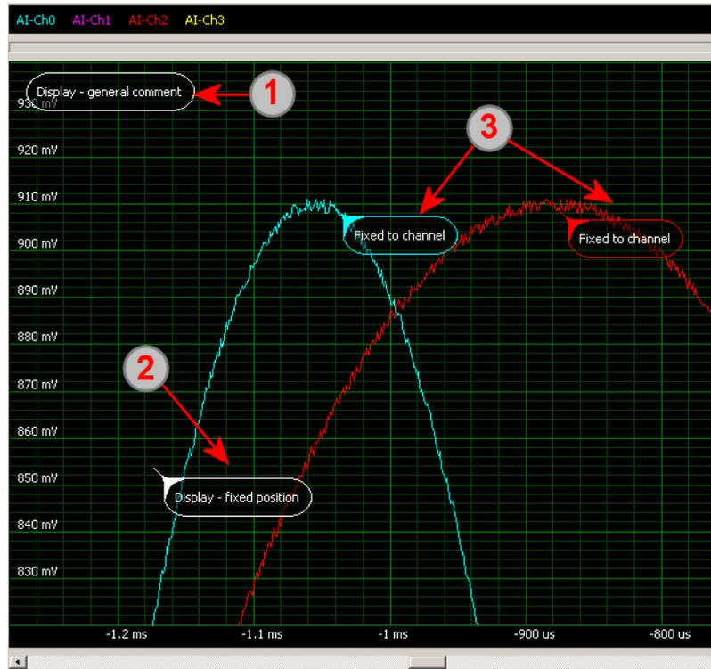
The display comments stay at the display even if a new acquisition is made. The channel comments are only valid for signal data they've been fixed to. If a new acquisition is done these comments are deleted as the data has changed.
