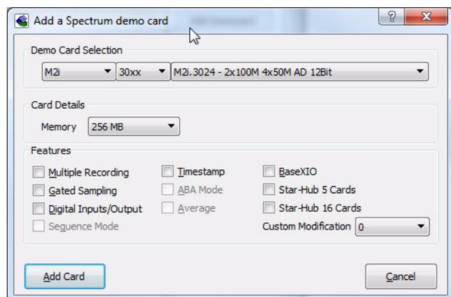
Installed demo cards are listed together with the real hardware in the main information tree as described above. Existing demo cards can be deleted by clicking the related button. The demo card details can be edited by using the edit button. It is for example possible to virtually install additional feature to one card or to change the type to test with a different number of channels.
