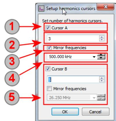
The harmonics cursor shows the normal cursor line as full line with a arrow marker at the bottom of the line. The number of harmonics is shown as dotted lines in the correct x axis position related to the current position of the main cursor.
