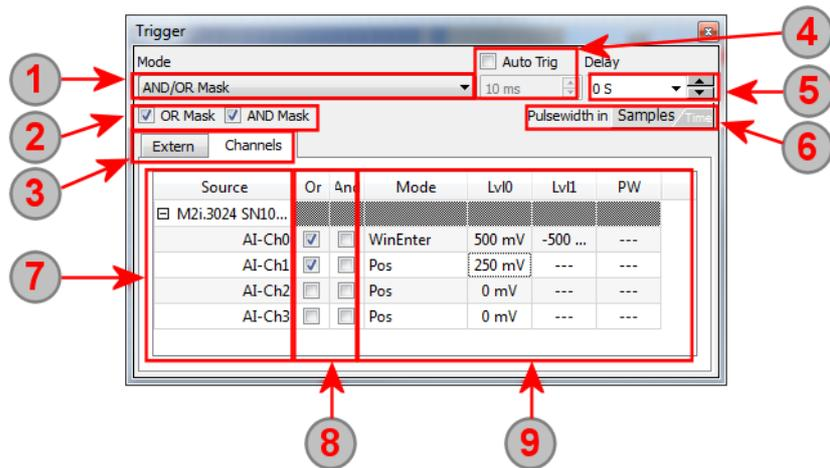
1 The general trigger mode allows to switch between software trigger, single hardware source or the versatile multiple hardware sources with AND/OR mask based trigger conjunction.
