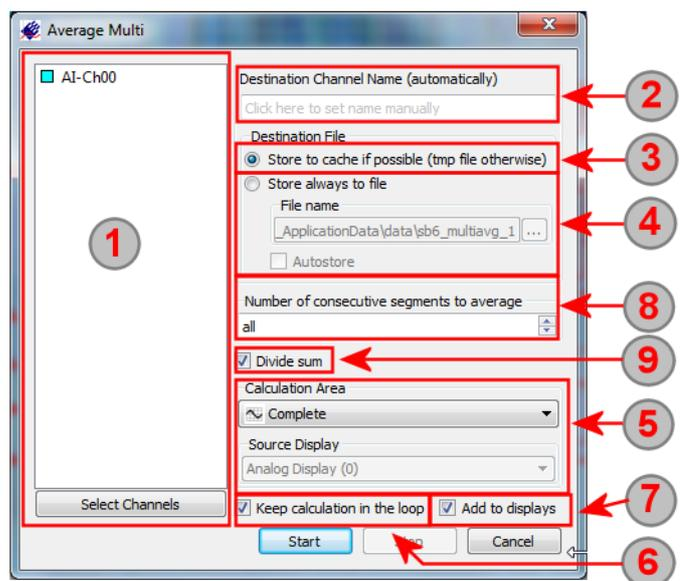
9 When checked the resulting average signal will be divided by the number of average loops and will therefore have the very exact resolution as the source signal.
