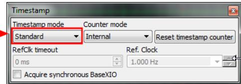
If Gated Sampling is activated the timestamp information is needed to show segmented information. Multiple Recording signals can also be shown without timestamp information just showing the segment borders with no time position information then.
