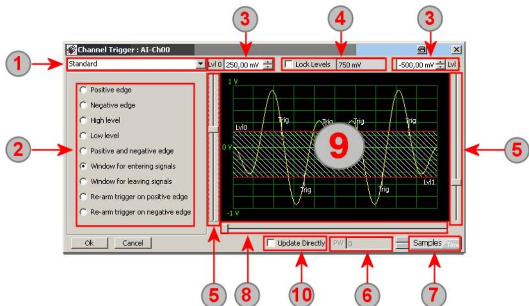
7 The Samples/Time button allows to switch between samples entry and time entry for the pulse width entry. When switching between the modes the currently selected value will be recalculated and shown in the new unit then.
