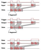
The Multiple Recording mode allows the recording of several trigger events without restarting the hardware. With this option very fast repetition rates can be achieved. The on-board memory is divided in several segments of same size. Each of them is filled with data if a trigger event occurs.
