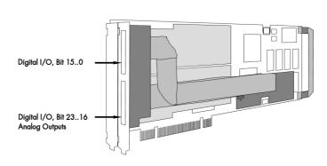
The additional inputs and outputs are mounted on an extra bracket. The figure shows the allocation of the two connectors.
