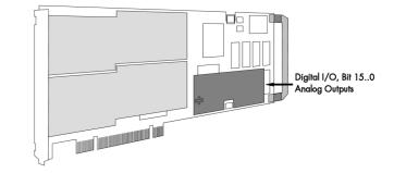
brakket, but are available on an internal connector. The figure shows the position of this connector on the bottom side of the extra I/O piggyback module.
