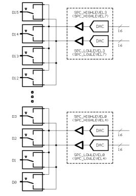
The minimum distance between a LOW level and its corresponding HIGH level for one output group is 100 mV. It is also not possible to program the LOW level of one group higher than its HIGH level. In both cases the software driver will return an error.
