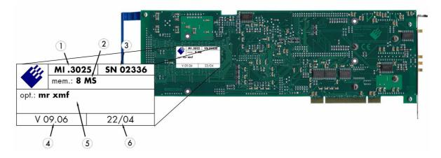
The Spectrum type plate, which consists of the following components, can be found on all of our boards.
