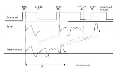
Due to the structure of the on-board memory there is another delay at the end of the gate interval.
