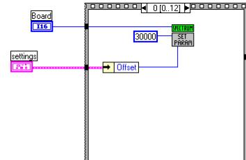
Changes the settings that could be changed while output is running. These are offset, amplitude and filter.
