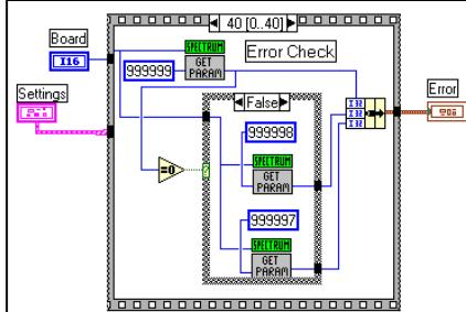
This VI writes the settings to the MI.61xx. If the settings are not changed this function must only be called one time. The parameters are set in a sequence. At the end of the sequence a check for errors is made. If an error has occurred the errorcode, the error generating register and the error generating value are given back. The registers are listed at the end of the document.
