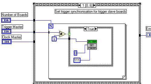
Starts two or more MI-boards for synchronization. To synchronize two MI boards the clock and trigger synchronization information is written in the correct order.
