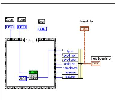
Initialises the installed boards and the software driver. The standard initialisation function of the driver is called and after that some data is read from the onboard EEPROM. The initialisation must be performed one time before any other commands are allowed to access the board.
