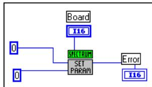
This VI makes a software reset of the board. The currently running replay stops immediately.
