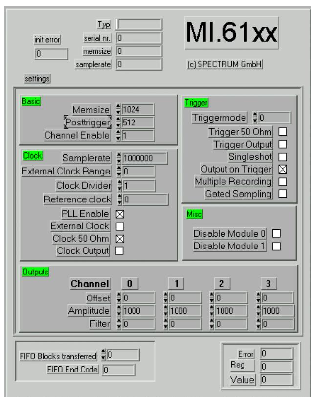
This VI shows the use of the FIFO mode with the MI.61xx boards under LabVIEW. After starting the VI, a simple sine signal is generated continuously with current parameters. In this example only channel 0 is used.
