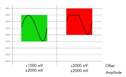
To avoid heavily distorted output signals please make sure to keep the signals in a range of ±3000 mV.
