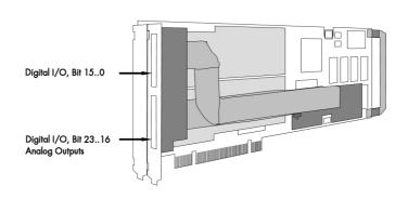
The additional inputs and outputs are mounted on an extra bracket.
