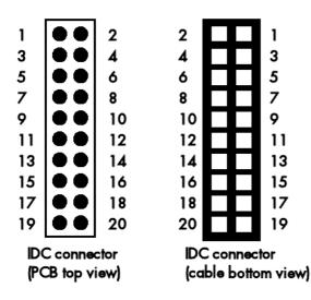
The 20 pole IDC connectors have the following footprints. For easy usage in your PCB the cable footprint as well as the PCB top footprint are shown here. Please note that the PCB footprint is given as top view.
