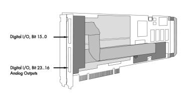
The additional inputs and outputs are mounted on an extra bracket.
