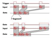
The Multiple Recording mode allows the recording of several trigger events without restarting the hardware. With this option very fast repetition rates can be achieved. The on-board memory is divided in several segments of same size. Each of them is filled with data if a trigger event occurs.
