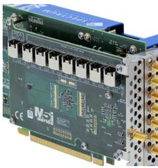
The Star-Hub is an additional module allowing the phase stable synchronization of up to 8 boards of a kind in one system. Independent of the number of boards there is no phase delay between all channels. The Star-Hub distributes trigger and clock information between all boards to ensure all connected boards are running with the same clock and trigger. All trigger sources can be combined with a
