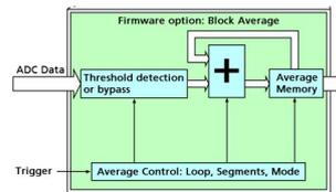
The Block Average Module improves the fidelity of noisy repetitive signals. Multiple repetitive acquisitions with very small dead-time are accumulated and averaged.
