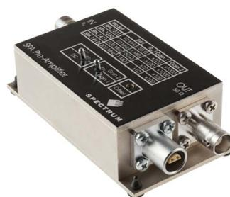
For the acquisition of extremely small voltage levels with a high bandwidth a series of external amplifiers is available. Each of the one channel amplifiers is working with a fixed input impedance and allows - depending on the bandwidth - to select different amplification levels between x10 (20 dB) up to x1000 (60 dB). Using the external amplifiers of the SPA series voltage levels in the  $\mu\text{V}$  and mV area can be acquired.
