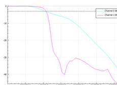
This option is only available for the M4i.3321-x16 (2 x 3.2 GS/s 12 Bit Digitizer with 1 GHz bandwidth). This option changes the hardware input filter of the card. The -inptd option optimizes the input stage for time domain measurement with a modified filter characteristic to minimize overshoot and undershoot on
