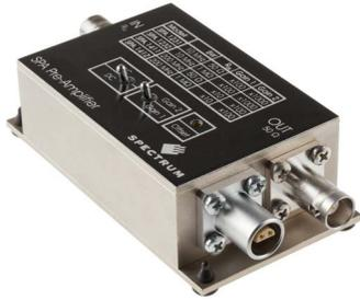
For the acquisition of extremely small voltage levels with a high bandwidth a series of external amplifiers is available. Each of the one channel amplifiers is working with a fixed input impedance and allows - depending on the bandwidth - to select different amplification levels between x10 (20 dB) up to x1000 (60 dB). Us-
