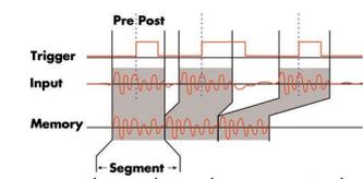
The Multiple Recording mode allows the recording of several trigger events with an extremely short re-arming time. The hardware doesn't need to be restarted in between. The on-board memory is divided in several segments of the same size. Each of them is filled with data if a trigger event occurs. Pre- and posttrigger of the segments can be programmed. The number of acquired segments is only limited by the used memory and is unlimited when using FIFO mode.
