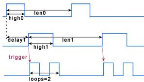
The digital pulse generator option adds 4 internal independent digital pulse generators with programmable duty cycle, output frequency, delay and number of loops.
