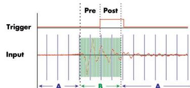
The ABA mode combines slow continuous data recording with fast acquisition on trigger events. The ABA mode works like a slow data logger combined with a fast digitizer. The exact
