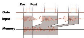
The Gated Sampling mode allows data recording controlled by an external gate signal. Data is only recorded if the gate signal has a programmed level. In addition a pre-area before start
