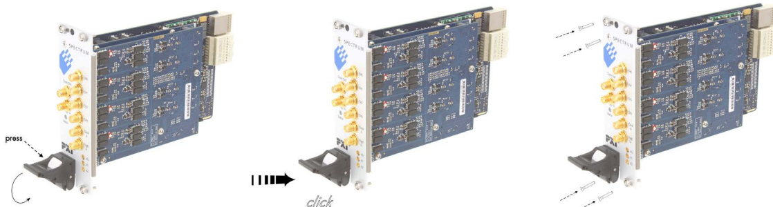
Image 9: Installation of PXle cards with connector handling and mounting screws
