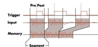
The Multiple Recording mode allows the recording of several trigger events with an extremely short re-arming time. The hardware doesn't need to be restarted in between. The on-board memory is divided in several segments of the same size. Each of them is filled with data if a trigger event occurs. Pre- and posttrigger of the segments can be programmed. The number of acquired segments is only limited by the used memory and is unlimited when using FIFO mode.
