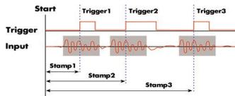
The timestamp function writes the time positions of the trigger events in an extra memory. The timestamps are relative to the start of recording, a defined zero time, externally synchronized to a radio clock, an IRIG-B or a GPS receiver.
