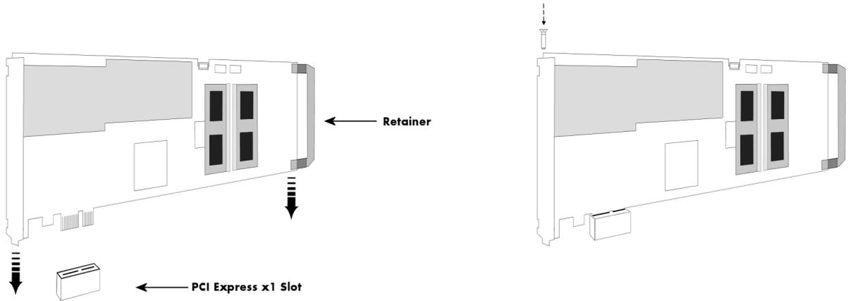
**Installing the M2i/M3i.xxxx-exp PCI Express card in a PCIe x4, x8 or x16 slot**
