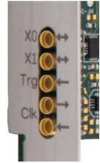
The multi purpose I/O lines are available on the front plate and labelled with X0 (line 0 = X0 = Ext1) and X1 (line 1 = X1 = Ext2). As default these lines are switched off.
