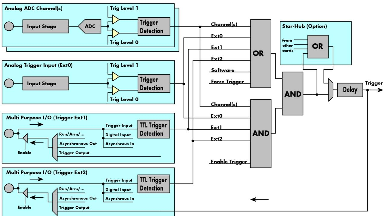
The trigger engine of the M3i card series allows to combine several different trigger sources with OR and AND combination, with a trigger delay or even with an OR combination across several cards when using the Star-Hub option. The above drawing gives a complete overview of the trigger engine and shows all possible features that are available.
