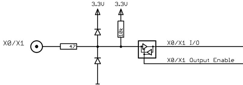
The maximum forward current limit for the used 1N4148 diodes is 100 mA, which is effectively limited by the used series resistor for logic levels up to 5.0V. To avoid floating levels with unconnected inputs, a pull up resistor of 10 kOhm to 3.3V is used on each line.
