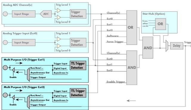
The M3i card series has two additional multi purpose lines that can be programmed as additional TTL trigger inputs to be combined either with the main (analog) external trigger or with some of the channel trigger modes explained later in this manual.
