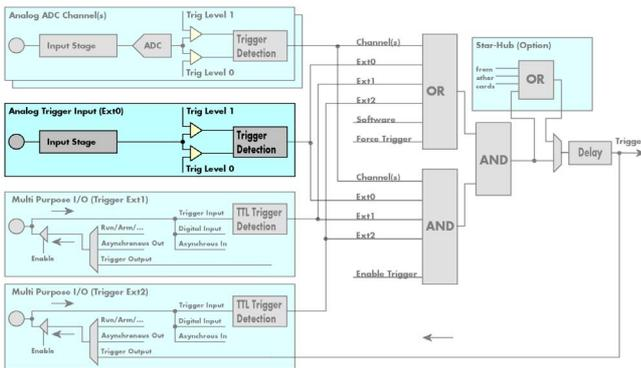
The M3i series has one main external trigger input consisting of an input stage with programmable termination and programmable AC/DC coupling and two comparators that can be programmed in the range of +/- 5000 mV. Using two comparators offers a wide range of different trigger modes that are support like edge, level, re-arm and window trigger.
