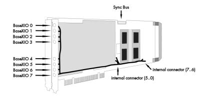
mounted on-board. To gain easier access, these lines are connected to an extra bracket, that holds eight SMB male connectors. For special purposes this option can also be ordered without the extra bracket and instead with internal cables.
