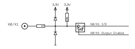
The maximum forward current limit for the used 1N4148 diodes is 100 mA, which is effectively limited by the used series resistor for logic levels up to 5.0V. To avoid floating levels with unconnected inputs, a pull up resistor of 10 kOhm to 3.3V is used on each line.
