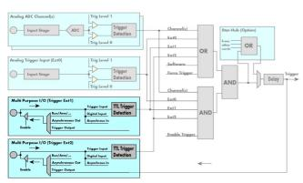
The M3i card series has two additional multi purpose lines that can be programmed as additional TTL trigger inputs to be combined either with the main (analog) external trigger or with some of the channel trigger modes explained later in this manual.
