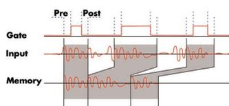
The Gated Sampling mode allows data recording controlled by an external gate signal. Data is only recorded if the gate signal has a programmed level. In addition a pre-area before start of the gate signal as well as a post area after end of the gate signal can be acquired. The number of gate segments is only limited by the used memory and is unlimited when using FIFO mode.
