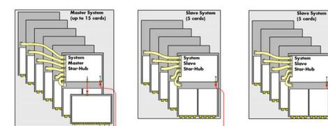
With the help of multiple system star-hubs it is possible to link up to 17 system phase synchronous with each other.
