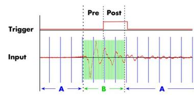
The ABA mode combines slow continuous data recording with fast acquisition on trigger events. The ABA mode works like a slow data logger combined with a fast digitizer. The exact
