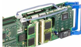
The star-hub is an additional module allowing the phase stable synchronisation of up to 16 boards in one system. Independent of the number of boards there is no phase delay between all channels. The star-hub distributes trigger and
