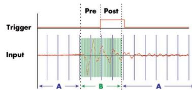
The ABA mode combines slow continuous data recording with fast acquisition on trigger events. The ABA mode works like a slow data logger combined with a fast digitizer. The exact position of the trigger events is stored as timestamps in an extra memory.
