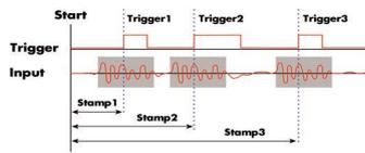
The timestamp function writes the time positions of the trigger events in an extra memory. The timestamps are relative to the start of recording, a defined zero time, externally synchronized to a radio clock, an IRIG-B a GPS receiver. Using the external synchronization gives a precise time relation for acquisitions of systems on different locations.
