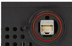
The GBit Ethernet connection can be used with standard COTS Ethernet cabling. The integration into a standard LAN allows to connect the digitizerNETBOX/generatorNETBOX either directly to a desktop PC or Laptop or it is possible to place the instrument somewhere in the company LAN and access it from any desktop over the LAN.
