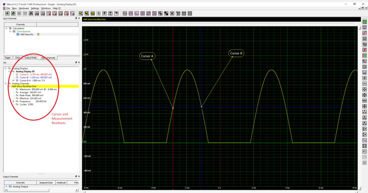
**Figure 3: Measurement example showing the use of cursor and a small sample of measurement parameters applied to a half wave rectified sine waveform.**
