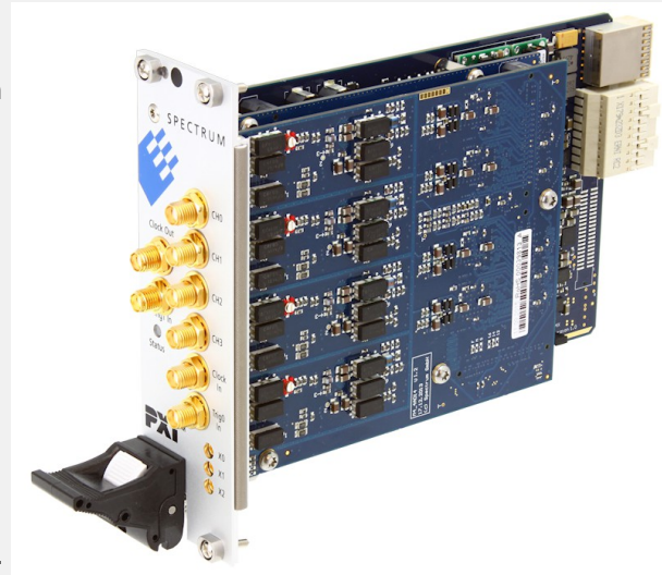
Figure 3: Spectrum M4x.4451-x4, 4 channel 500 MS/s 14 bit digitizer with PXIe interface
