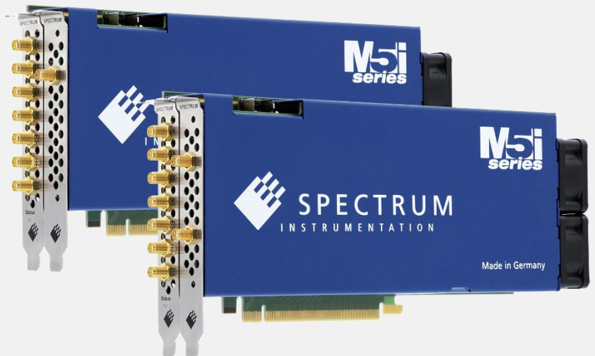
Figure 1: New M5i.3360-x16 (1 channel) and M5i.3367-x16 (2 channel) leading bandwidth digitizers by Spectrum Instrumentation combine 10 GS/s sampling, 12-bit resolution, 4.7 GHz bandwidth, and 12.8 GB/s data streaming.
