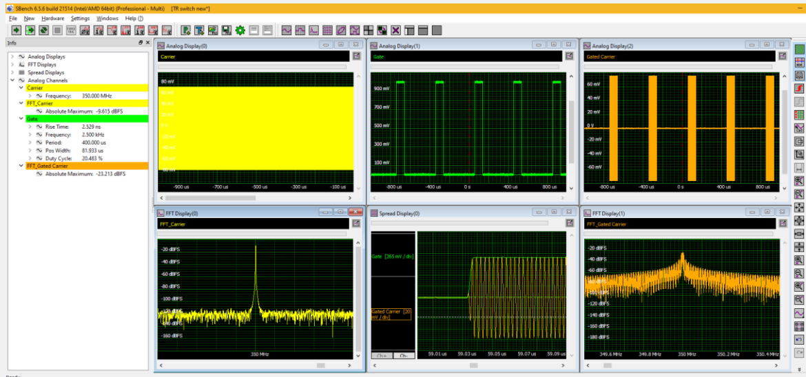
Figure 4: Analysis of a T/R switch RF input (upper left grid), gate signal (upper center grid), and the T/R switch output (upper right).
