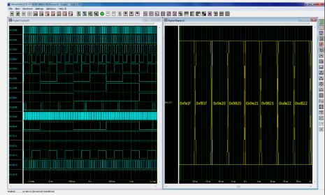
The 32-bit wide Digital I/O the parallel digital buses as shown in figure 5.
