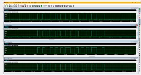
Figure 10: Any of these four different Manchester encoded serial data packets stored in the AWG waveform memory can be selected for output under computer control while the previous packets is being output. The selected packet is output as soon as the current pack
