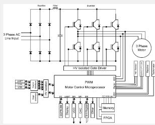
Figure 2: A typical motor control system uses pulse width modulation to control a three-phase motor. The control system is a mixed signal device using analog and digital signals
