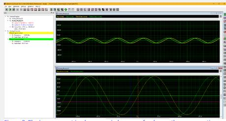
Figure 8: The improvement in phase margin because of a change the compensation network values. The delay is -17.91 µs and the unity gain frequency has shifted to 6.304 kHz and the phase margin is now a more stable -40.6°.
