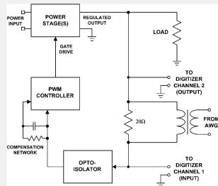
Figure 6: The functional block diagram of a switched mode power supply showing the introduction of a small perturbing signal to measure the phase margin of the power supply control loop.
