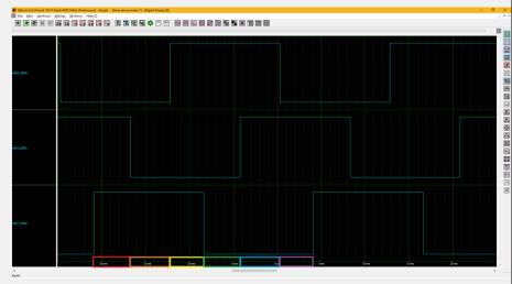
Figure 4: The three phases of the hall effect sensor allow the controller to determine the motor rotational speed as well as the shaft's angular position.
