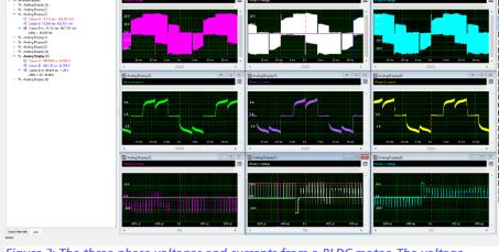
Figure 3: The three phase voltages and currents from a BLDC motor. The voltage The acquisition duration of waveforms are shown in the top row, currents in the middle row, and a zoom view of the voltage waveforms in the bottom row.
