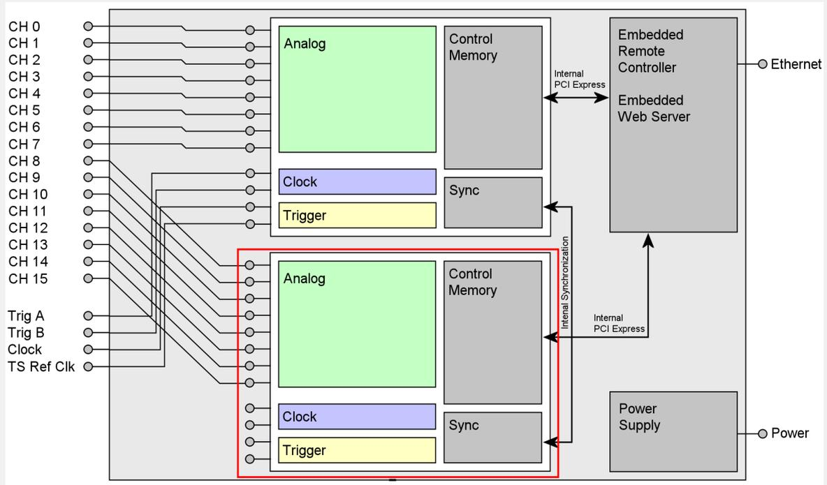
**Figure 2: The block diagram of a 16 channel digitizerNETBOX showing the principle components including multiple digitizers, power supply, and embedded controller.**
