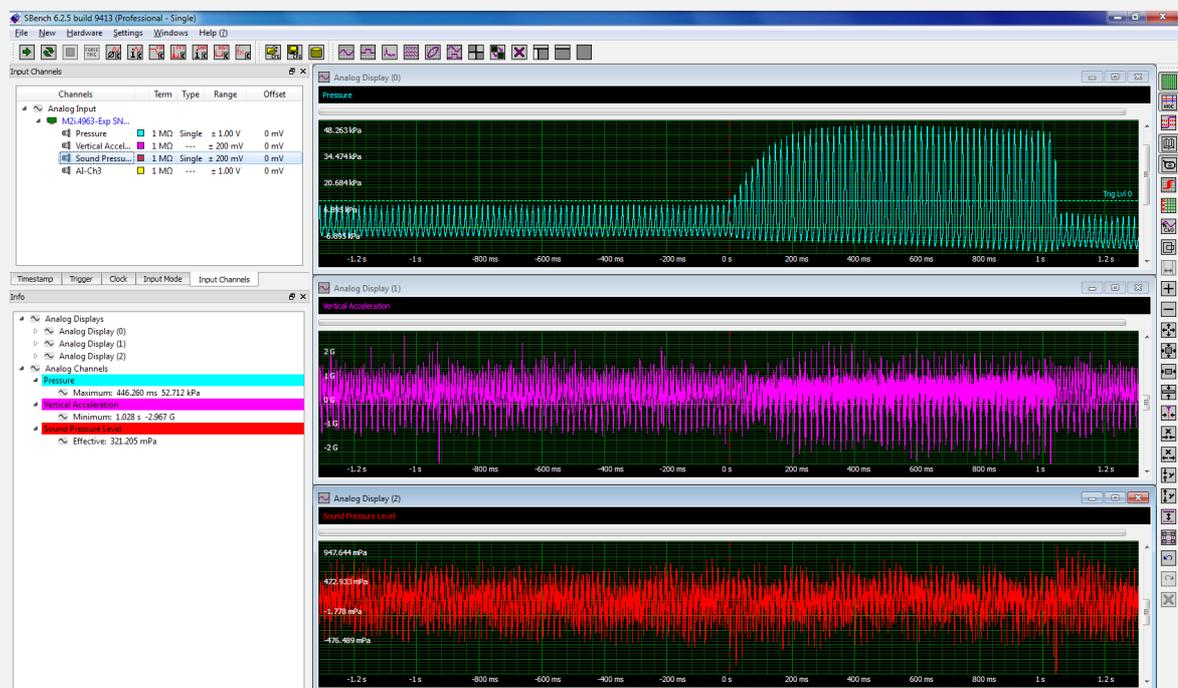
Figure 4: The SBench 6 screen showing the results of a measurement of the maximum pressure of the air compressor. The top grid is the pressure waveform. The middle grid is the vertical vibration acceleration, and the bottom grid is the sound pressure level.
