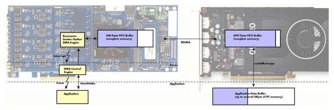
Buffer handshaking for DMA transfer from Spectrum Digitizer to GPU (or vice versa) using RDMA uses the same registers as the transfer from Digitizer to host (or host to Generator) as described in the "Buffer handling" section of the hardware manual.
