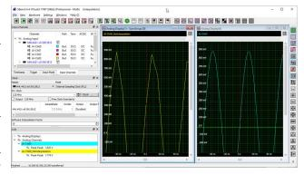
trace on the right is the same signal but with interpolation activated. Both traces have been expanded vertically so you can examine the top of the sine wave. Parameter measurements for the Peak to Peak amplitude (lower left corner) made for both traces show the significant improvement in amplitude accuracy that's possible.
