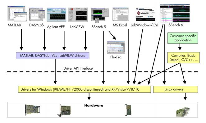
The Spectrum drivers offer you a common and fast API for using all of the board hardware features. This API is nearly the same on all operating systems. Based on this API one can write your own programs using any programming language that can access the driver API. This manual detailed describes the driver API allowing you to write your own programs.
