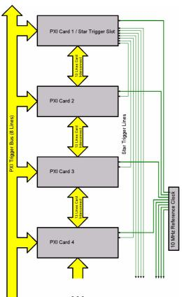
The defined additional PXI lines shown in the drawing on the left allow the easy synchronization of multiple cards without needing additional external components or cables. With some restrictions it is also possible to synchronize PXI cards from different manufacturers using the special PXI features of the boards.
