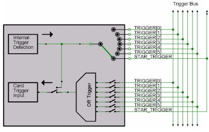
As soon as the PXI trigger output register is programmed, this internal trigger will not be used for triggering the card itself, but is routed to the programmed PXI line. The figure is showing all of the possible PXI trigger connections.
