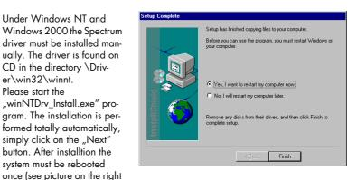
side). The driver is install to support one PCI/PXI or CompactPCI device. If more boards are installed in the system the configuration of the driver has to be changed. Please see the following chapter for this topic.
