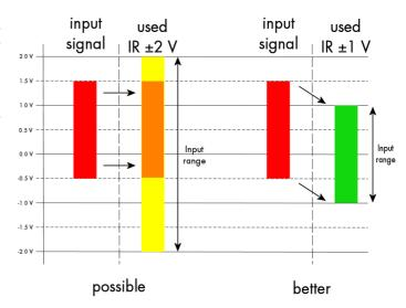
The example in the right figure shows signals with a range of  $\pm 1.0$  V that have offsets up to  $\pm 1.0$  V. So related to the desired input range these signals have offsets of  $\pm 100$  %.
