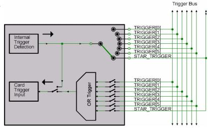
As soon as the PXI trigger output register is programmed, this internal trigger will not be used for triggering the card itself, but is routed to the programmed PXI line. The figure is showing all of the possible PXI trigger connections.
