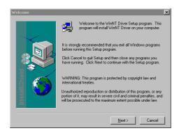
Under Windows NT and Windows 2000 the Spectrum driver must be installed manually. The driver is found on CD in the directory \Driver\win32\winnt. Please start the "winNTDrv\_Install.exe" program. The installation is performed totally automatically, simply click on the "Next" button. After installtion the system must be rebooted
