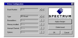
The Windows NT lagacy driver must be configured by the Driver Configuration utility to support more than one board. The Driver Configuration utility is automatically installed with the driver. The Utility can be found in the start menu as "DrvConfig".
