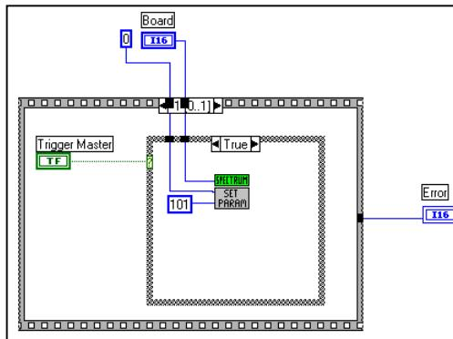
The VI Sync is used to synchronise several boards with each other. This VI will only transfer the synchronisation information. All other settings and the start of the board is done as described before. If only one board is present in the system this function need not to be used.
