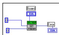
This VI makes a software reset of the board. The currently running recording stops and data in memory is not valid.
