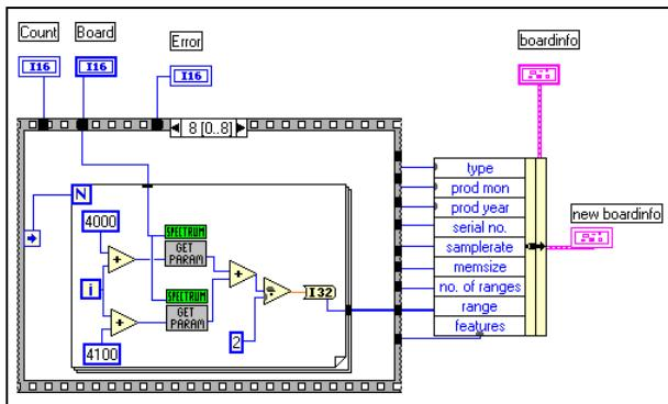
Initialises the installed boards and the software driver. The standard initialisation function of the driver is called and then some data is read from the onboard EEPROM. The initialisation must be performed one time before any other commands are allowed to access the board.
