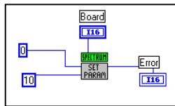
This VI starts the board with the current settings. If the settings are not changed they don't need to be programmed again before starting the board.
