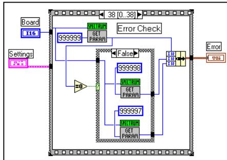
This VI writes the settings to the MI.31xx. If the settings are not changed this function must only be called one time. The parameters are set in a sequence. At the end of the sequence a check for errors is made. If an error has occurred the errorcode, the error generating register and the error generating value are given back. The registers are listed at the end of the document.
