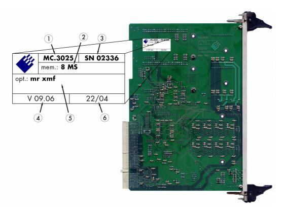
The Spectrum type plate, which consists of the following components, can be found on all of our boards.
