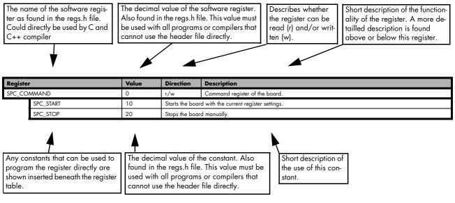
If no constants are given below the register table, the dedicated register is used as a switch. All such registers are activated if written with a "1" and deactivated if written with a "0".
