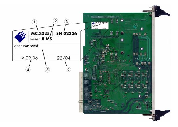
The Spectrum type plate, which consists of the following components, can be found on all of our boards.
