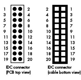
The 20 pole IDC connectors have the following footprints. For easy usage in your PCB the cable footprint as well as the PCB top footprint are shown here. Please note that the PCB footprint is given as top view.
